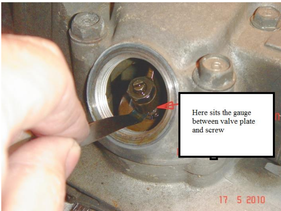
Figure 6: one feels the valve clearance
