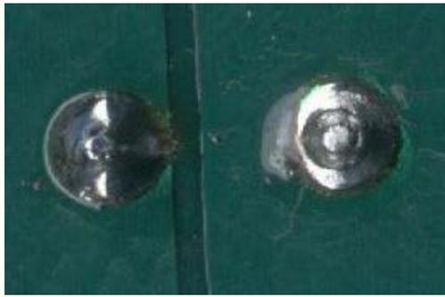
On the left is a good joint. It is bright and shiny and smooth. On the right is the curse of any circuit, a dry joint, note the obvious ring around the wire, this is in fact a crack in the solder caused by either vibration or electrical loading resulting in heat. You can also make out the satin finish on the solder as apposed to the bright smooth appearance on the good joint on the left.
