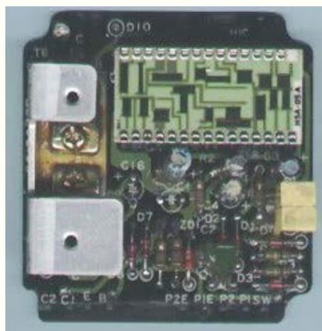
Inside the left hand unit there is a Printed Circuit Board (PCB'd) that is held in by 3 screws and a line of soldered connections down the edge (red box) that connect the board to the sockets where the wiring plugs into the case. The right hand one has the edge solder and two screws through the back of the case.
